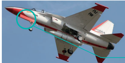
Landing Gear Door
