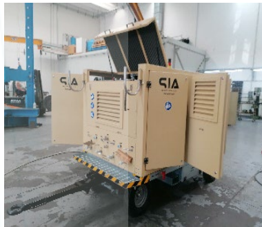
Skydrol hydraulic bench for ATR 42/72 double-line aircraft
