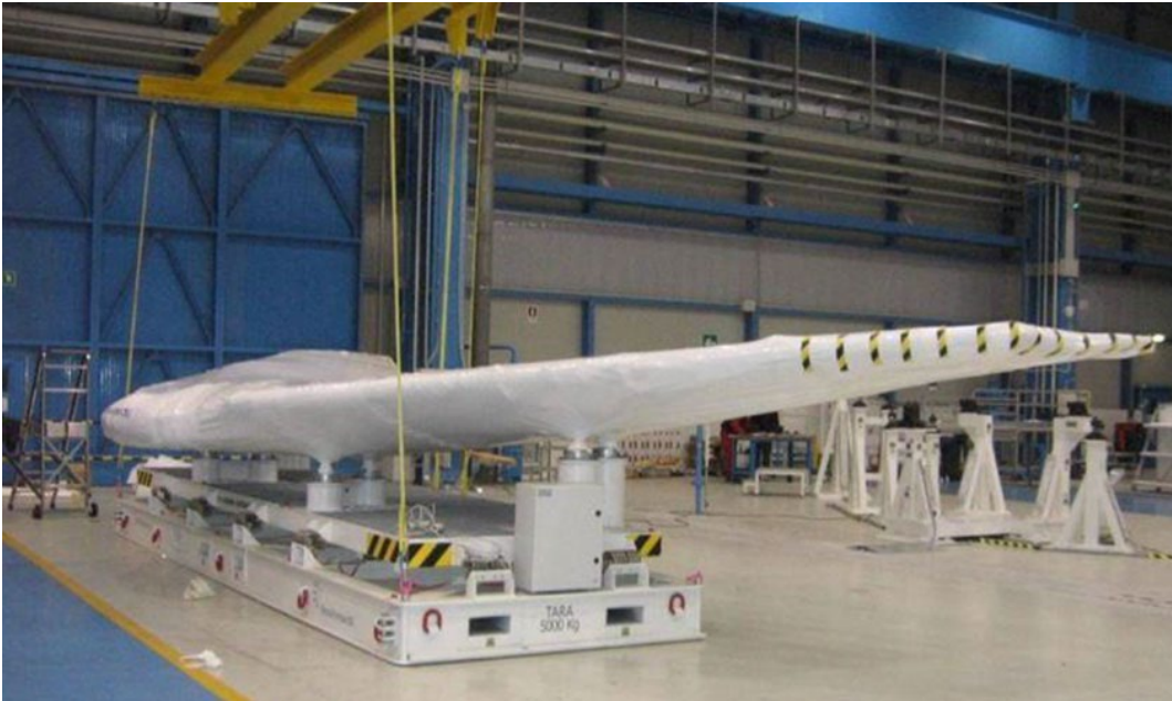
Tool for transporting (in flight configuration) by air or sea the Horizontal Stabilizer of the Bombardier C-Series aircraft
